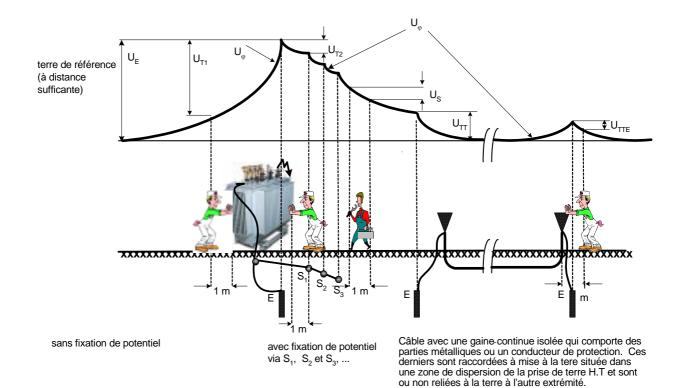
reference earth (at sufficient distance)
