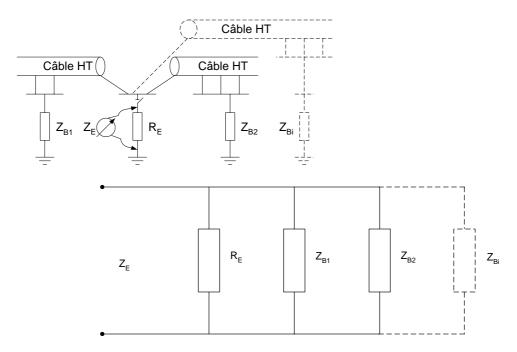
**Loop impedance of an earth connection** " $Z_{EB}$ ": impedance of the circuit made up of the resistance " $R_E$ " of the earth connection in series with the impedance " $Z_B$ " which constitute all the other earth return paths.
